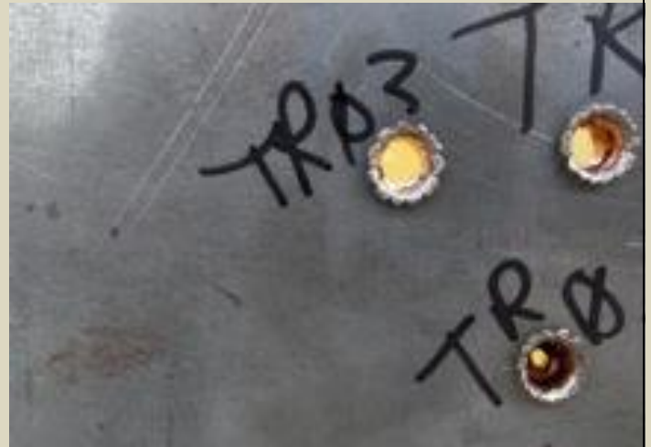
Figure 2 ND 4.6 x 30 mm vs. 3/16" NATO Steel
